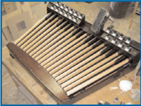
(Top) Pedal board with new maple key tops and toe studs. (Bottom) Painstaking and exacting pipe making at the Russell shop in Vermont.
